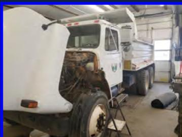
This rig had a couple of gauges not working. While making the repairs we installed a new block heater and a new hour meter. We also found a bad u-joint while inspecting the rig.
