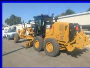
Left: We took possession of our new 140M2 Road Grader with just 3600 hours. It is a very nice machine! We are installing a company radio, lights and new cutting edges.
