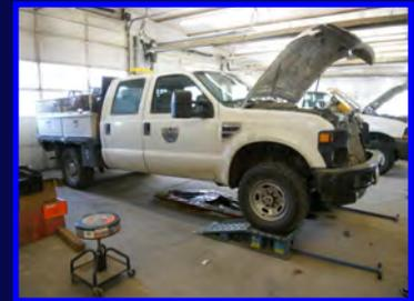
We pulled the hydraulic cooler, cleaned it, and straightened the fins.
