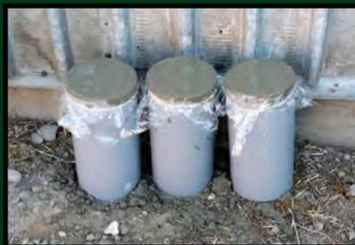
The approach portion of the "C" Street alley concrete work was completed earlier this week. Three cylinders were cast for strength testing to help determine when to open the alley for vehicular traffic.
