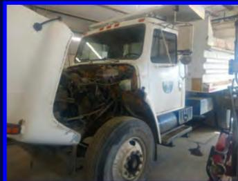
We are adjusting clutches, clutch brake and checking over the dump trucks for chip seal.
