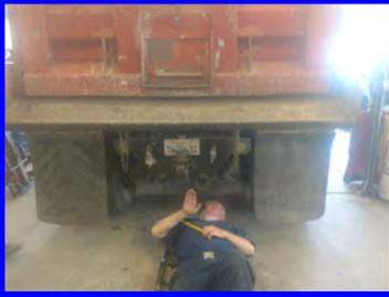
We are building a new rear hook so we can hook up to the chip spreader for chip seal.
