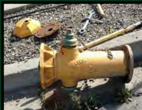
A fire hydrant was replaced on Orchard Street. It broke during hydrant flushing work.
