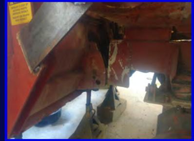
This chip spreader is in for some much needed repairs. We started by pulling off the distributor head and replacing the pins and building up the mounts. We will also be working on the hydraulics.
