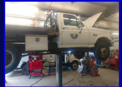
Right: The rear fuel tank pump went out. We are replacing the pump and fuel tank selector switch.
