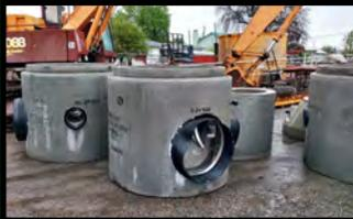
Parts for the 3 large water manholes arrived this week. The inside of each manhole base is precisely shaped as to allow water to flow through each manhole with minimum turbulence.
