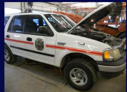
We installed new front and rear brakes and rotors. We also installed a toggle switch to turn off the back up beeping mechanism.
