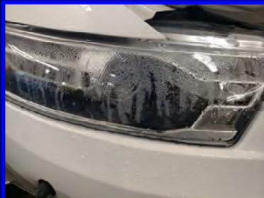
We pulled apart the front of the car to drain the water and reseal the headlight assembly.
