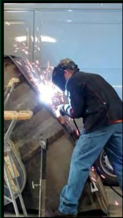
Left: Brian worked to apply a “hard face” surface on the wear edges of the crusher bucket.
