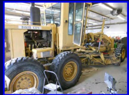
We installed the snow wing on the grader so the plow crew can pull away the snow from driveways and intersections.
