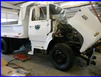
We are repairing the transmission and replacing the carburetor on this plow for the airport.
