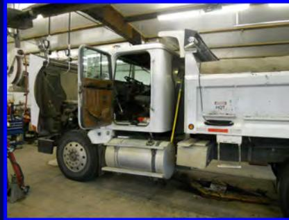
We replaced the foot brake valve and this rig is back to work.
