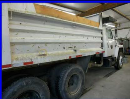
The tailgate pin fell out and bent the mount on one side. We straightened it and reinstalled.
