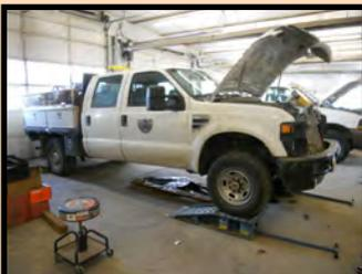
Scott replaced the front hubs and front brakes.
