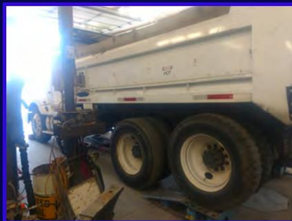
We replaced the leaky rear axle and installed a Speedy Sleeve. This rig is back in service.
