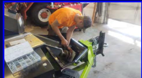
We fabricated a chunk of plastic to stop gravel from coming out while operating.
