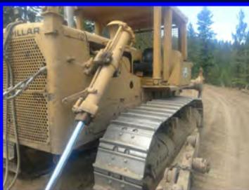
Left: We re-welded a new pin mount for the C-frame on this dozer.
