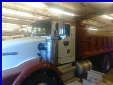
We installed some interior plastic molding and shortened the body dump lever.
