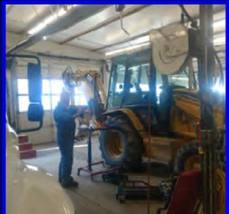
Right: Here you see Scott replacing the self-leveling solenoid on this equipment.
