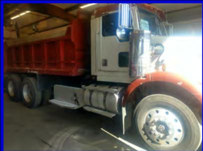
Left: This rig got a new fuel sending unit and new LED cab lights and turn signals.
