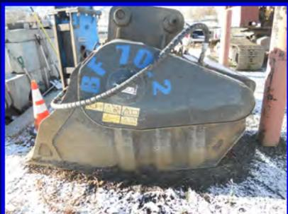
Left: The crusher bucket received a new spring and anvil and is back in service.
