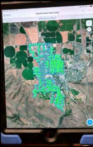
Nate and Riley continue to make good progress opening and closing water valves in zones 1 and 2. The green dots represent those valves that have been “exercised” and the blue circles with the yellow “X” inside still need to be done.
