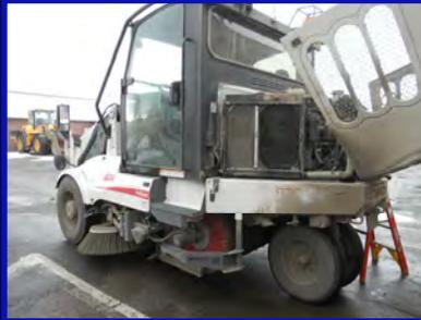
The drive belt and motor sprocket came apart. We replaced the sprocket and tightened the chain. This truck is back in service.
