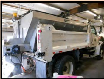
We replaced the flipper blades and a hydraulic line on this rig. We also mounted the sander.
