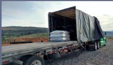
A tarp system was used to protect the pipe while in transit.
