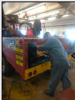
Work continues on the chip spreader. Both belts that feed gravel to the front were replaced as well as the rubber shields that hold the gravel in the bed.
