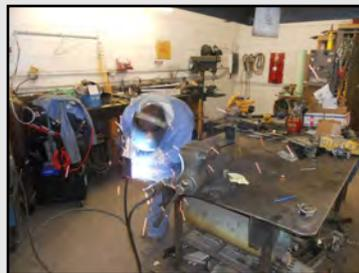
Pictured above, Nate is building light brackets for the Fire Department's Type III fire truck. These brackets will be mounted at a later date.
